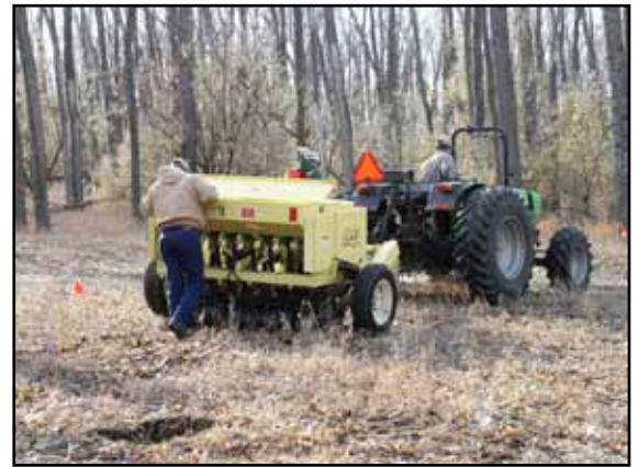
Seeding with a no-till drill into chemically fallowed sod
