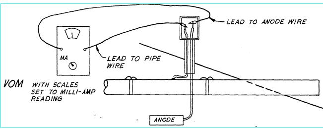
The following basic equipment is needed for maintenance testing:
