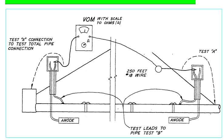
Test "A" will show if the pipe is making a continuous circuit.
