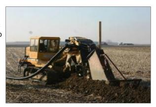
Subsurface drainage is used in areas having a high water table where the benefits of lowering the water level are worth the expense. The practice also applies to areas that will benefit from controlling groundwater and surface runoff. The soil must meet certain suitability requirements and an adequate outlet must be available to assure proper drain function.
