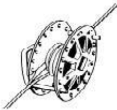
Figure 1. This is an example of an in-line tensioner.
