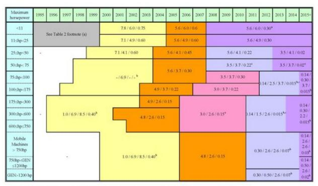
a) The PM standard for hand-start, air cooled, direct injection engines below 11 hp may be delayed until 2010 and be set at 0.45 g/bhp-hr.
