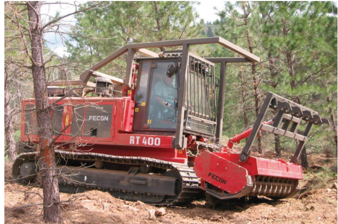
Figure 7 - Mastication equipment grinds vegetation into small debris creating a fire safe fuel profile, organic material for soil health improvement, and avoids burning debris and the associated air quality, fire hazard and pest breeding issues.
