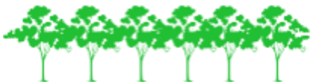
Figure 8a: Windbreak with reduced density in lower crown allowing wind and snow to blow through into areas needing protection.
