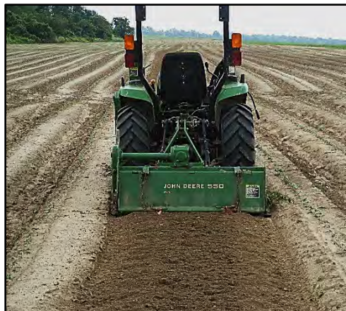
Figure 4: Preparing a seedbed with a 5-ft wide rototiller.
