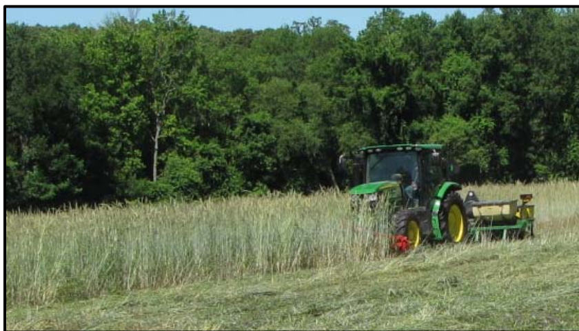
Figure 2: A front-mounted roller crimper allows simultaneous cover crop termination and cash crop planting.
