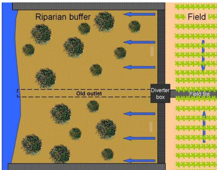
*Figure 1. Not-to-scale schematic of a riparian buffer with an intercepted tile outlet, diverter box, and distribution lines in the upstream part of the buffer (from Jaynes and Isenhart, 2011). Typically the old outlet will remain in place to outlet high flows that exceed the utilization capacity of the buffer.*
