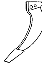
Figure 69 – Subsoiler (ripper) shank—Material section and shape that permit working depths greater than that of heavy duty chisel shanks or other primary tillage implements
