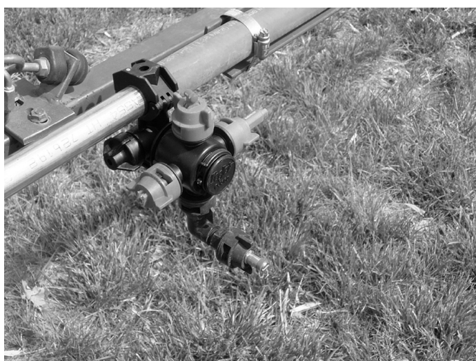
Figure 9. Multiple nozzle body on wet boom.
