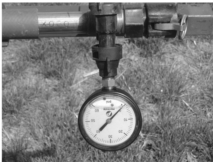
Figure 10. Gauge to check spray pressure on a wet boom.
