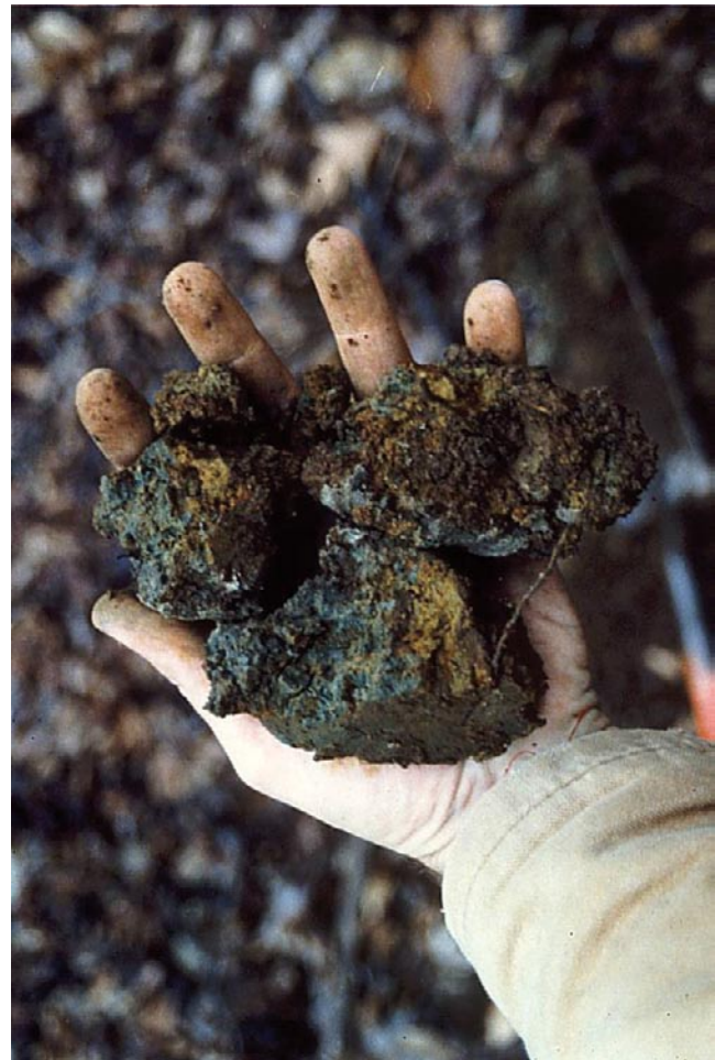
Figure 49. —Glaucconitic soils typically have gleyed, green or black matrices and can have mottles of weathered sulfides that can be mistaken for redox concentrations. If the weathered sulfides in this glauconitic soil were mistaken for redox concentrations, this nonhydric soil would appear to meet the requirements of indicator F6 (Redox Dark Surface).
