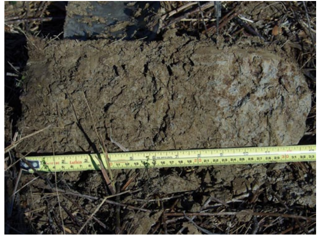
Figure 4. —This soil profile could meet the requirements of indicator F3 (Depleted Matrix); however, above the indicator, chroma is higher than 2 in a layer more than 15 cm thick. Only 15 cm of a chroma higher than 2 is allowed above an indicator.
