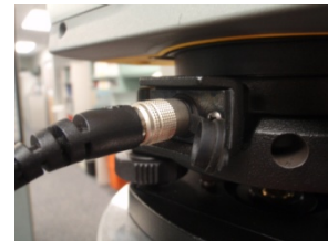
Figure 10: Battery connection to Total Station.
