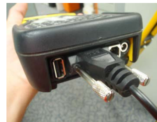
Figure 11: Battery connection to TSC2 Data Collector
