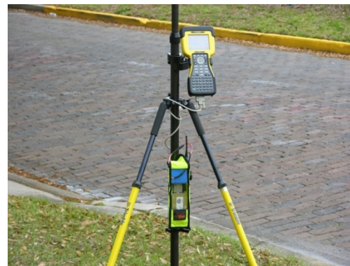
Figure 32: Complete set-up of VRS Network
