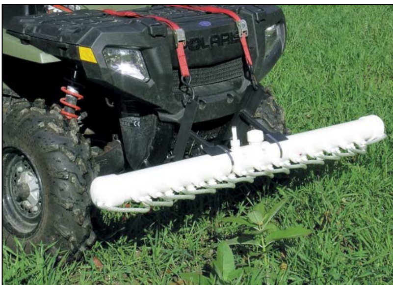
Small low impact herbicide rope wick applicators direct herbicide applications to target weeds without drift or overspray. These can be purchased or constructed for small ATV's or for commercial farm equipment.
