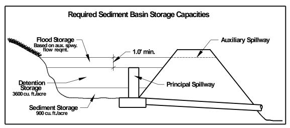
Flood storage is based on the required design storm for the auxiliary spillways. Flood storage is calculated between the crest of the principal spillway and the crest of the auxiliary spillway. A minimum of 1 foot in elevation is required between the principal and auxiliary spillways.
