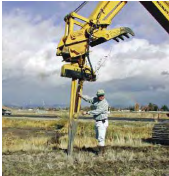
Figure 32: The use of a stinger for vegetative plantings (nativerevegetation.org).
