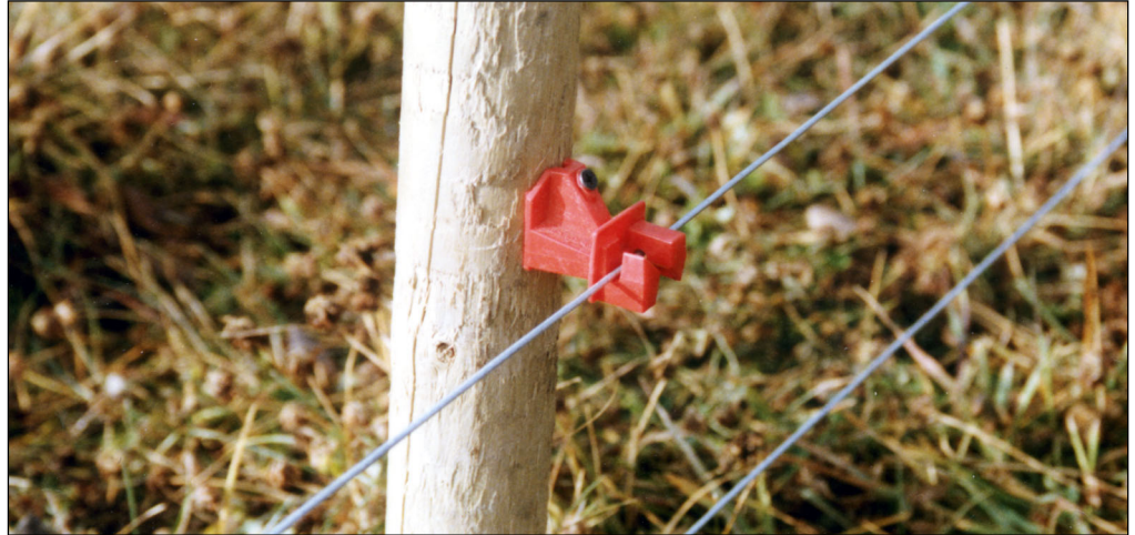
Figure 2 Typical Line Post Insulator
