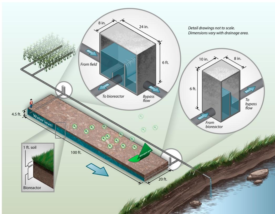
Figure 1. Schematic of a denitrifying bioreactor for agricultural drainage (From Christianson and Helmers, 2011)
