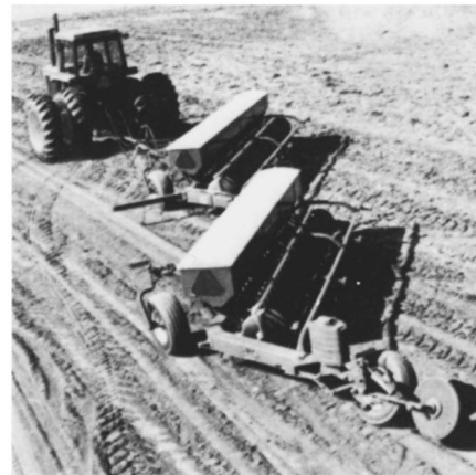
Figure 12 – One-way disk harrow—Equipped with seeder attachment—Squadron, wheel-mounted pull hitch
