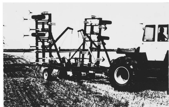
Figure 19 – Chisel plow—Dual folding wings—Wheel-mounted pull hitch
