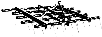
Figure 42 – Harrow—Section, round-wire teeth
