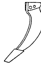
Figure 69 – Subsoiler (ripper) shank—Material section and shape that permit working depths greater than that of heavy duty chisel shanks or other primary tillage implements
