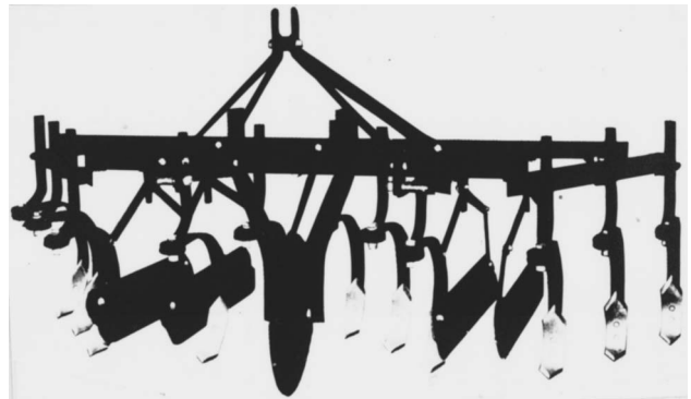
Figure 39 – Row crop cultivator—Same as Fig. 38 except two-row, rolling coulter for lateral stability
