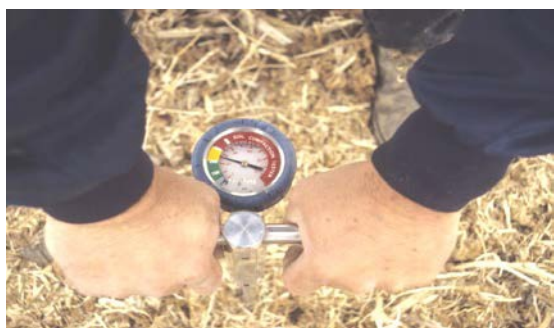
A soil penetrometer is one tool to check soil compaction depth. Source: NRCS Grigar Midland County
