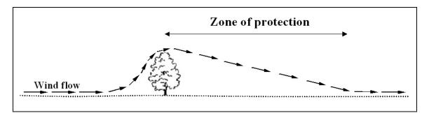
Research has shown that barriers significantly reduce wind speed for a distance of about 10 times the height of the barrier, in effect, reducing the field length along the erosive wind direction. However, the fully protected zone of any barrier diminishes as wind velocity increases and as the wind direction deviates from perpendicular to the barrier.
