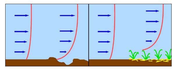
The nature of the surface over which the wind is traveling can greatly influence this wind profile, as well as the wind energy near the surface.
