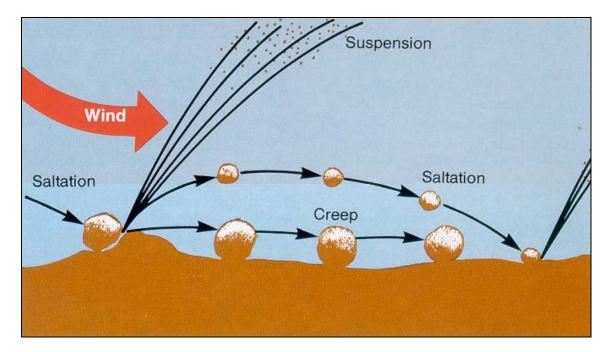
Under SURFACE CREEP, the force of the wind causes soil particles to roll along the soil surface until the wind slows, they are stopped by other particles, or they are trapped in a sheltered location, such as a furrow or a vegetated area. Surface creep generally involves
