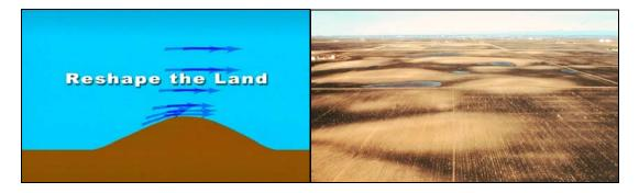
Reshaping the land by leveling knolls and benching slopes to shorten the unsheltered distance is an option in wind erosion control, but is usually not economical or practical. Because land reshaping is very costly, other effective control measures, such as no-till or seeding to permanent grass, are usually more viable options.
