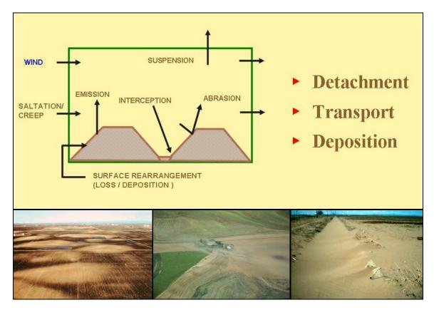
DETACHMENT occurs when the wind force against soil particles increases enough to overcome the force of gravity. Once detached, moving particles may collide and detach other particles.
