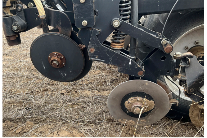
Figure 12. A single-disc (left) or double-disc (right) drill is often needed to implement a high-residue, no-till management system, and to successfully seed into tall, standing residue. Photos: USDA-NRCS.
