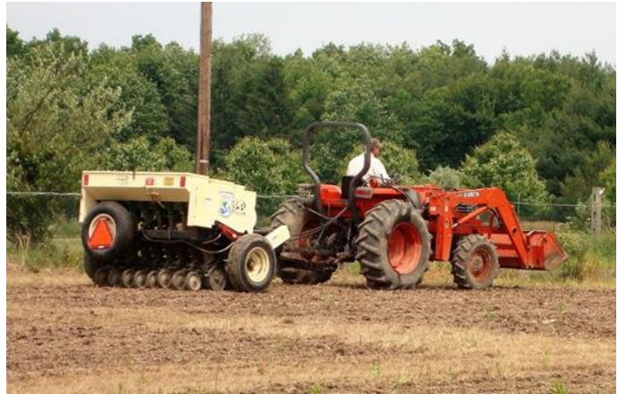
Figure 4.2. Native seed drills are ideal for large planting sites (5+ acres). Typical models have depth controls for optimal seed placement and separate seed boxes for different sizes and types of seed. Photos: Xerces Society/Kelly Gill.
