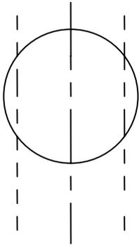
**Figure 1.** Single tile line or ditch passes through wetland and is unlikely to affect the hydrology of the entire basin in a normal 14 days.
