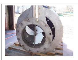
Screen with propeller drive for rotating the screen cylinder past brush during cleaning.
