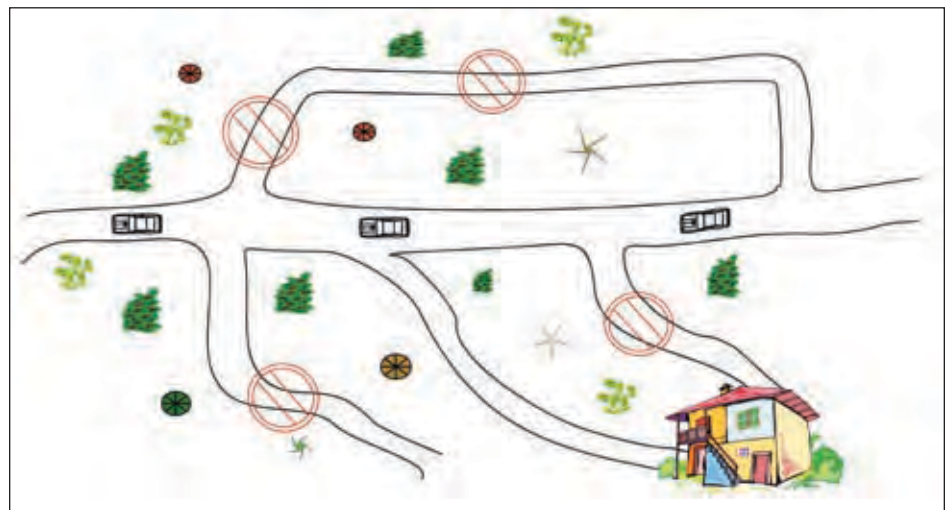
Figure V-6: Reduce road density. Close or remove multiple roads serving the same destination.
