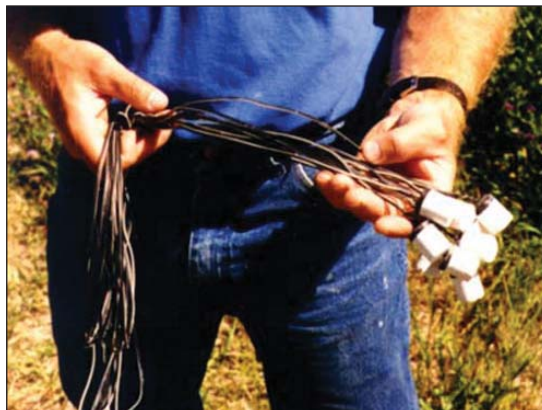
Gypsum blocks. NCAT photo.
