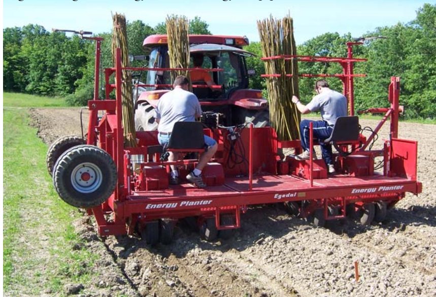
Figure 8: Egedal Energy willow energy crop planter built in Denmark
