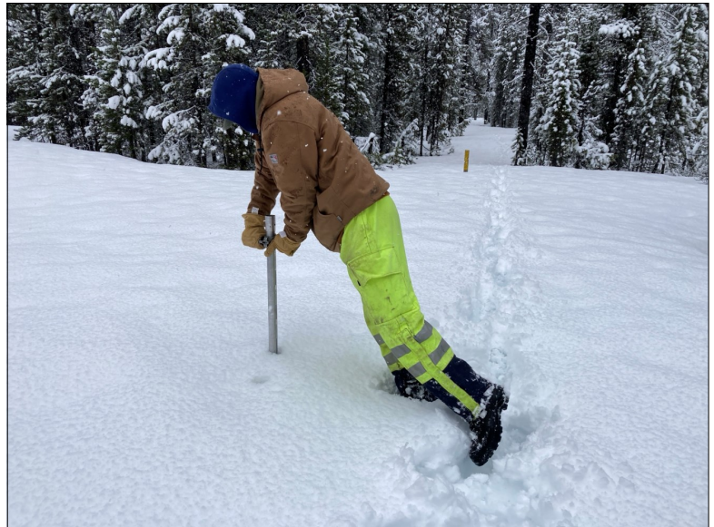
Coby Pope, PacifiCorp Hydro Repairman, driving through ice layers at North Umpqua Snow Course. Snowpack at the site is 221% of median as of April 1st.
