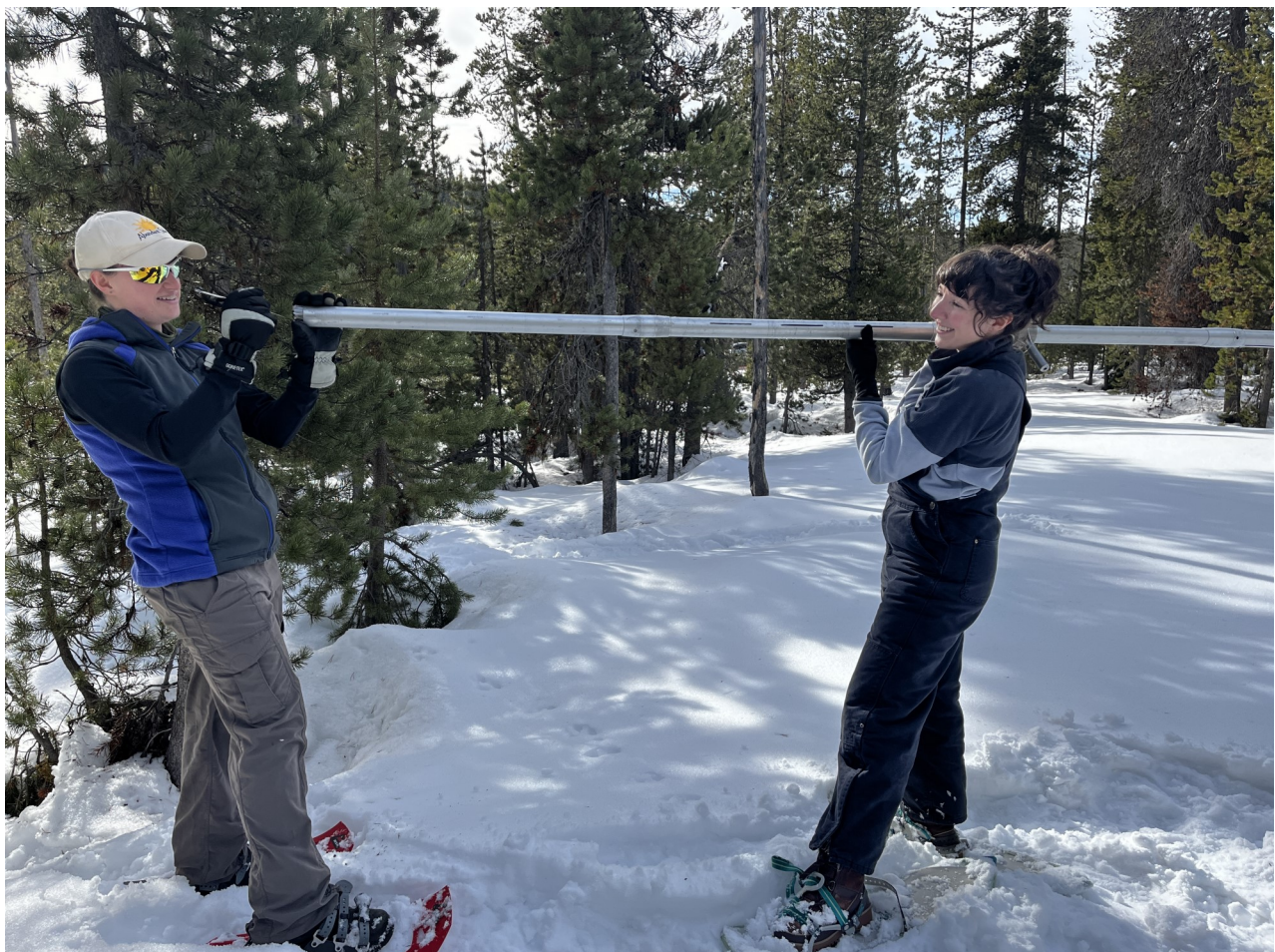
Julianne Robinson and Anna Burton, NRCS Engineers, prepare a snow core sample taken at the Tangent snow course east of Mount Bachelor. Snowpack at the site is 95% of median as of February 1st.
