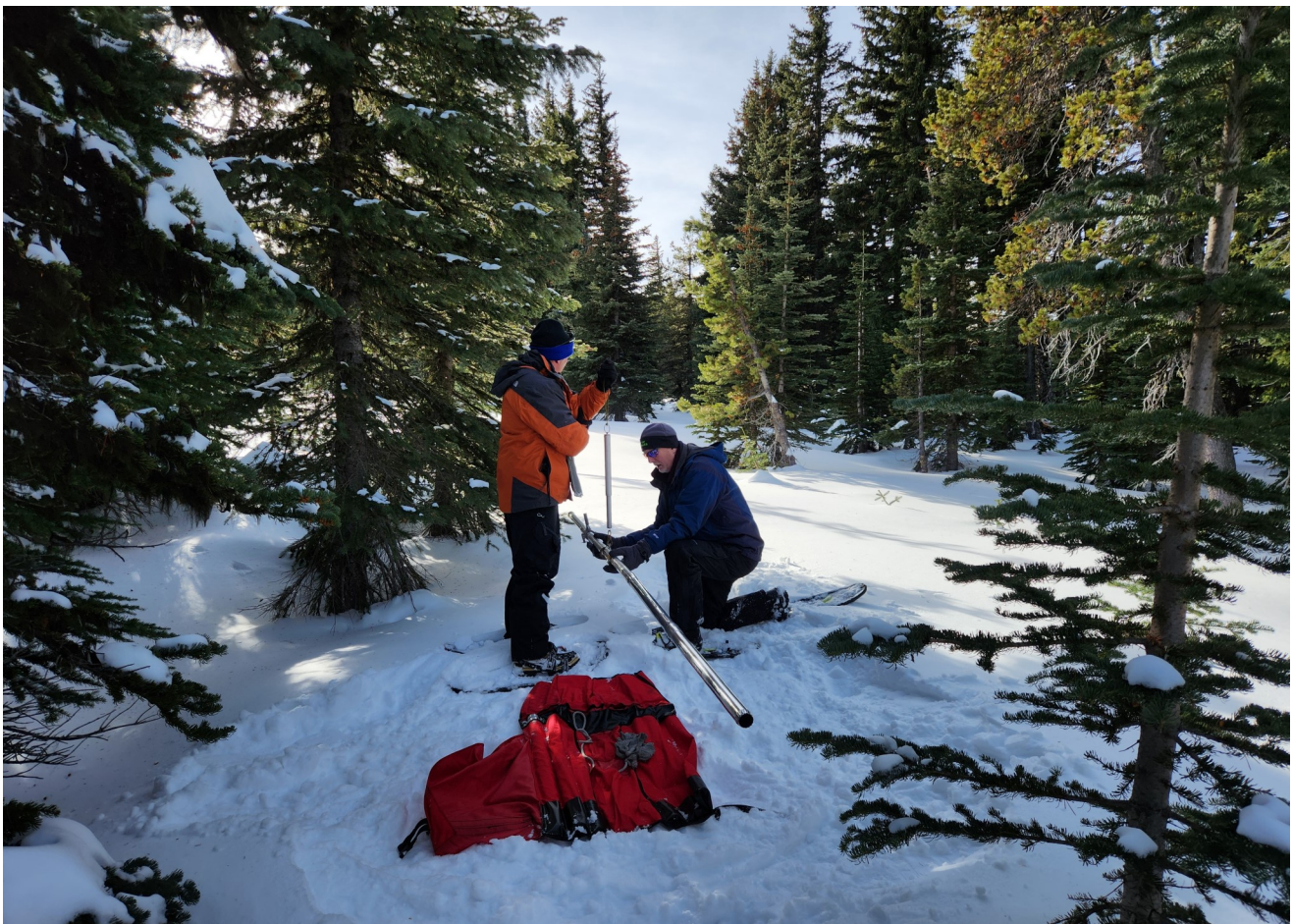
Dave Anderson and Dale McCabe, City of The Dalles, weigh a snow core sample along the High Prairie snow course. Dave Anderson has been measuring High Prairie snow course for over 30 years. Snowpack at the site is 84% of median as of February 1. Photo taken by Allen Buckman, NRCS Hydrologist (January 31, 2023)
