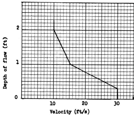
Avoid channel slopes between 0.7 and 1.3 of the critical slope except for short transition sections. Restrict supercritical flow to straight reaches.
