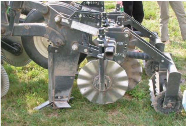
Figure 16.8. Left: A zone-tillage tool with hilling disks and rolling basket to create a zone of loosened soil. Right: Strip tillage also results in a narrow tilled zone that leaves most of the soil surface undisturbed. Photos by Robert Schindelbeck.
