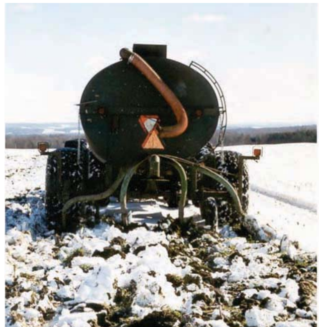
Figure 12.2. Injection of liquid manure into shallow frozen soils, which eliminates compaction concerns and reduces spring application volumes. Photo by Eleanor Jacobs.
