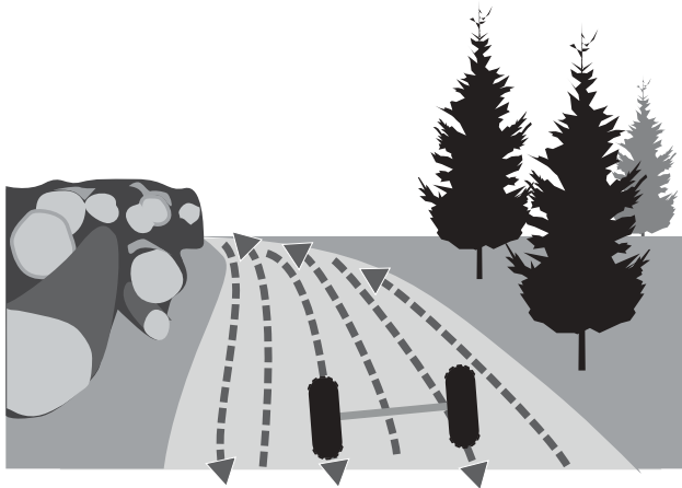
Figure 4-11. Splitting wheel or cat tracks when spreading and placing fill material to obtain additional compaction.
