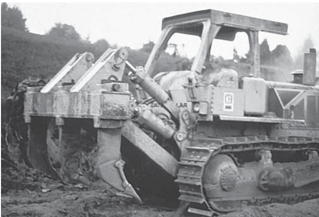
Figure 4-8. Tractor with a hydraulic ripper attachment.
